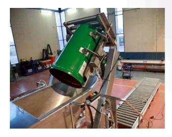
The unloading ramp feeds a tank which contains an agitator/crusher which breaks the product into pieces.
