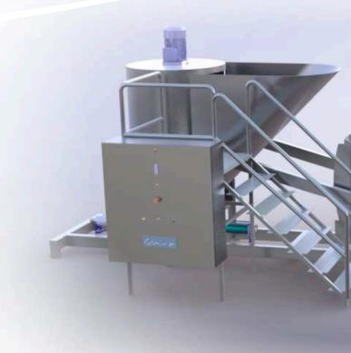
As the product turns into a liquid, a positive displacement lobe rotor pump with a feed screw sends the product to the heater, which completes the thawing of the product.
